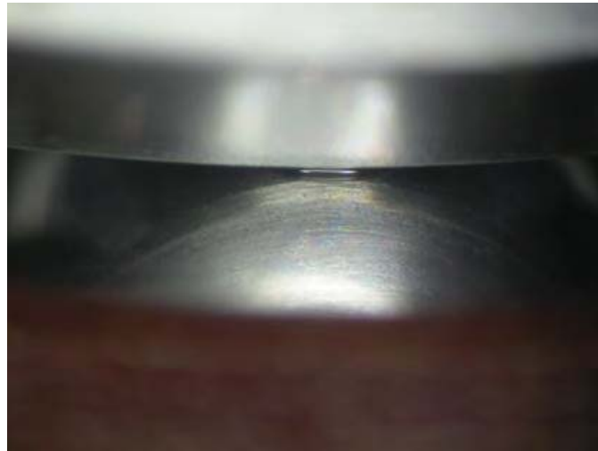
Figure 2. An impregnated phenolic cage with just an adequate amount of oil to show a small meniscus at start.
