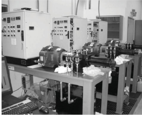
Figure 1. Rolling contact fatigue testers at The Aerospace Corporation.
