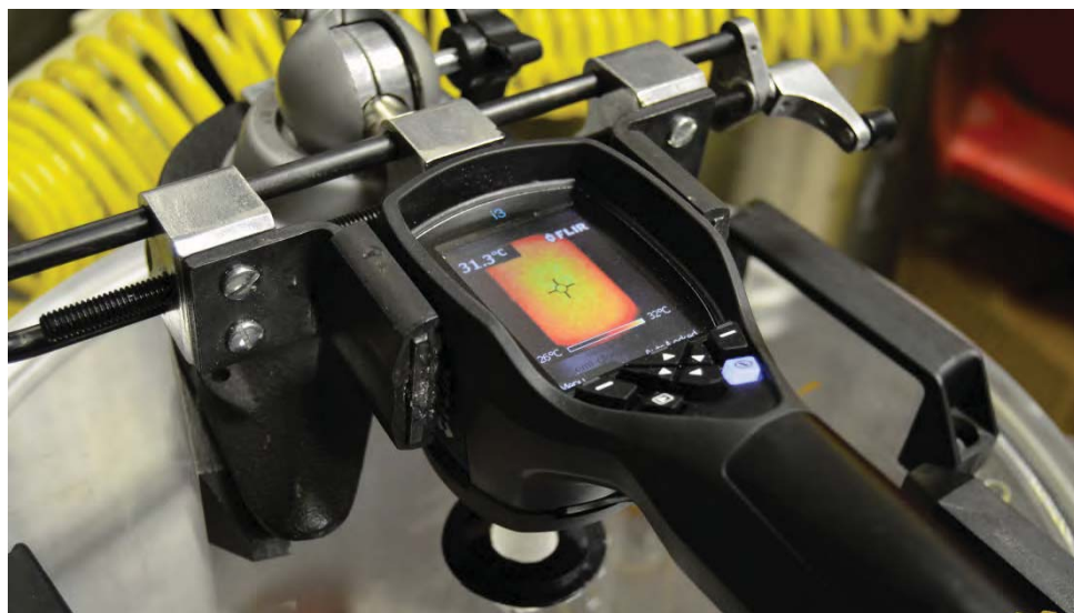
Figure 4. Thermographic (FLIR) instrument positioned above \text{CaF}_2 port in top of chamber.
