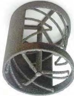
Figure 3. Build failure due to warping of slender flexures.
