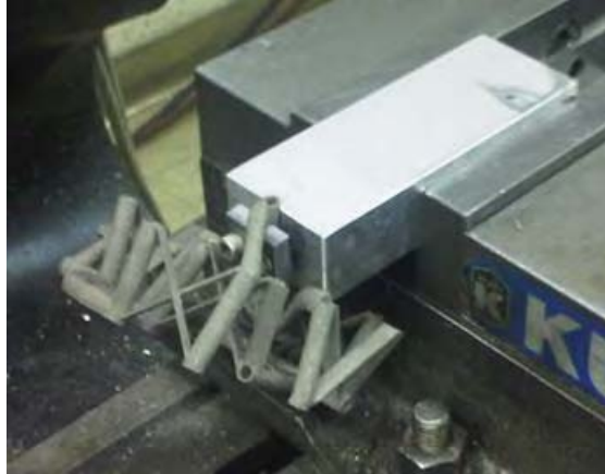
Figure 4. The 2 DOF pointer mechanism in fixture for removal of powder and supports from inside a split-tube flexure.
