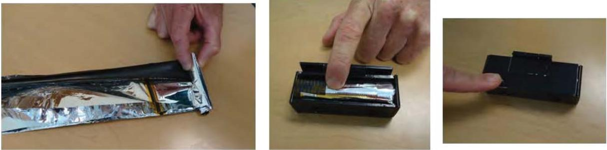
**Figure 6. Stowage of 3U CubeSat RODEO™ model**
