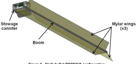
Figure 5. 3U CubeSat RODEO™ configuration
