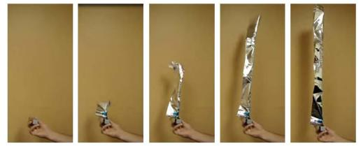
Figure 7. Deployment progression for 3U CubeSat RODEO
