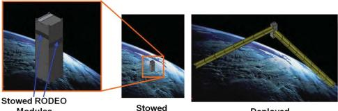
ModulesStowedDeployedFigure 1. 3U CubeSat with two Roll-Out De-Orbiting modules (RODEO™)
