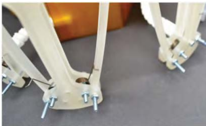
Figure 3. Torsion springs were affixed to the truss to bias the truss open
