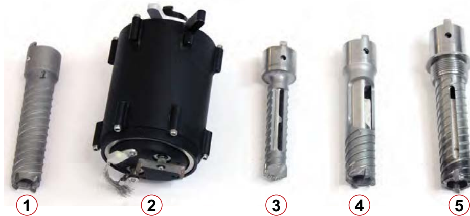
Figure 11. ROPEC Drill End Effectors (1) Standard Coring Bit (2) Rock Abrasion Brushing Bit (3) Powder and Regolith Acquisition Bit (4) Core PreView Bit (5) Slot Bit
