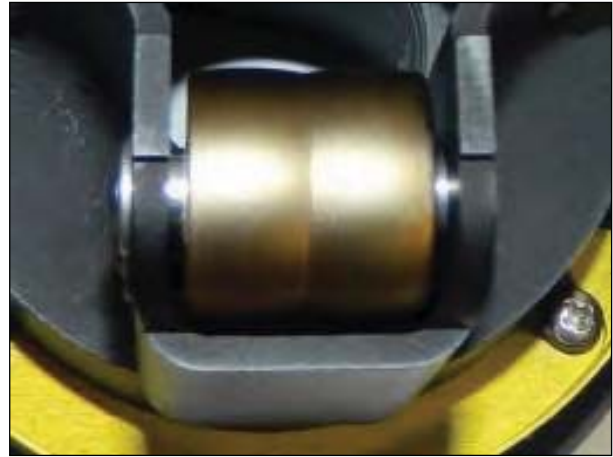
Figure 8. Side view of the guide wheel roller, clearly showing the Nedox coating, and the two curved contact surfaces for maintaining near line contact with the bit shank
