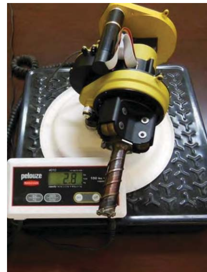
Figure 1. Weigh-in picture of the final mechanical assembly of the RANCOR drill
