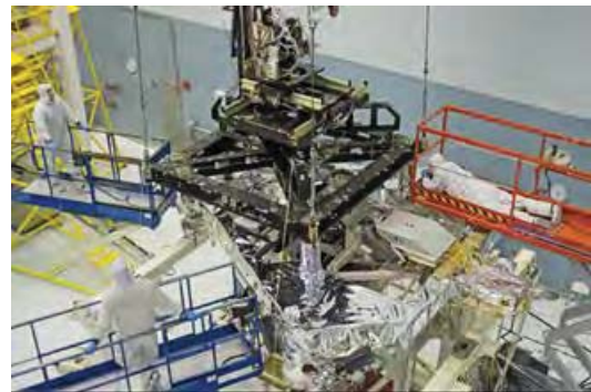
Figure 3. OSIM Bench being lowered into the SES Figure 4. OSIM during Ambient Alignment
