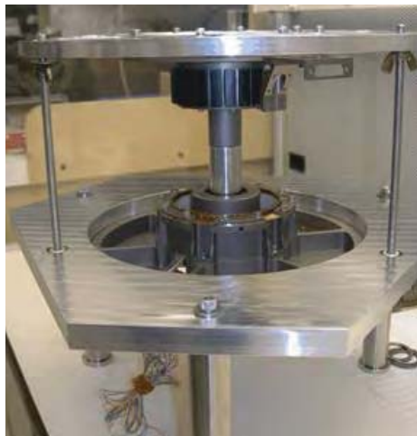
Figure 10. Motor Rotor Manually Lowered into Stator Assembly
