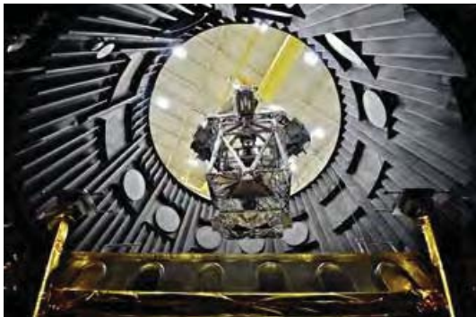
Figure 3. OSIM Bench being lowered into the SES Figure 4. OSIM during Ambient Alignment
