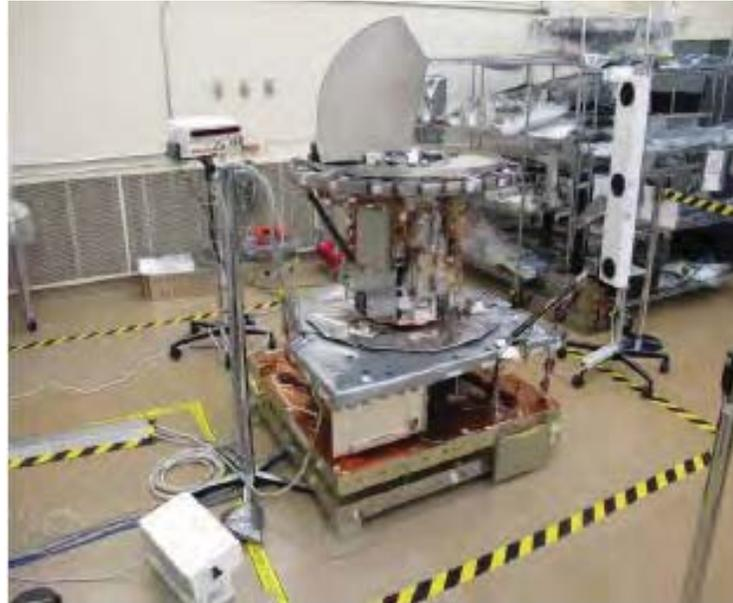
**Figure 1. Dynamometer Assembly Setup in Calibration and GMI without RDA and MR Assemblies Integrated**
