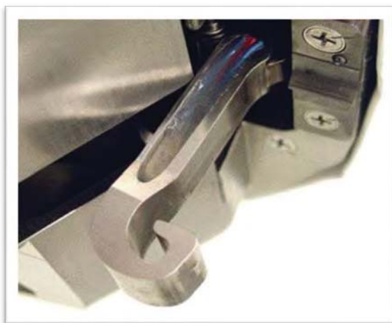
Figure 3. Base point and engagement hook of end effector
