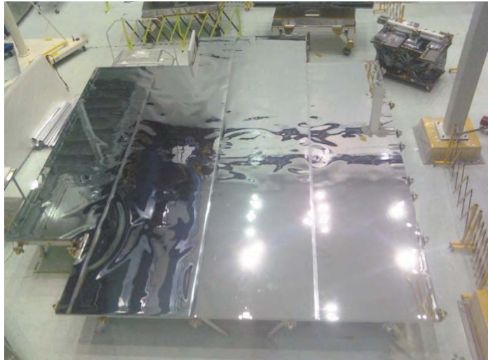
Figure 21. G-negation Table with Melinex 515 and Poron 4701-30
