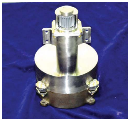
Figure 3. SSRMS LEE Snare Gearbox, Scale: OD = 4.86 inches (0.123 m) (Courtesy of MDA Corp)
