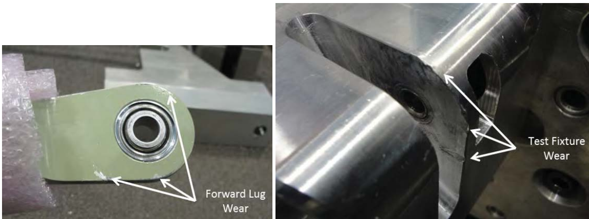
Figure 11. Wear Post-Vibration Testing (Forward Lug [left]; Test Fixture [right])
