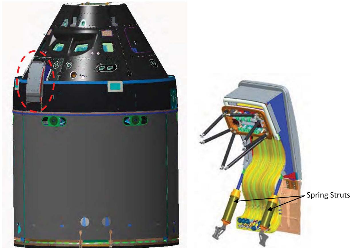
Figure 1. MPCV EFT-1 CM-SM Umbilical in its Stowed Configuration
