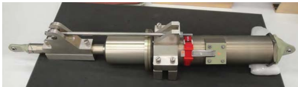
Figure 3. CM-SM Umbilical Spring Strut with Retention Tool
