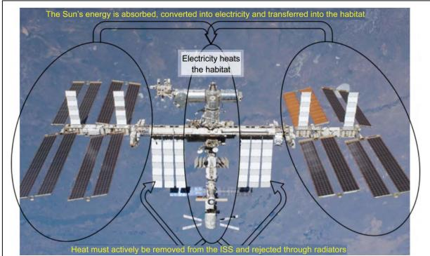
Figure 1. Thermal Control and Energy Balance of the International Space Station
