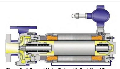
Figure 3. A Canned Motor Rotor with Centrifugal Pump, Typical of Actively Pumped Thermal Control Systems for Space Applications.
