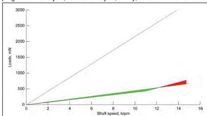
Figure 6. Hydrodynamic Load Capacity for the Rear Bearing on the Failed Pump. Green and Red Ranges Indicate Bearing Margin with Respect to the Lubricant Jet Force.
