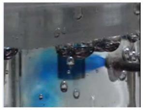
Coherent jet Impacts stub shaft Spreads to engage entire shaft area Potentially high pressure loads
