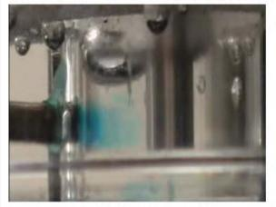
Low velocity jet breaking apart Diffusion dominated Moderate/low pressure loads
