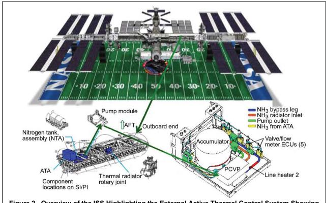
Figure 2. Overview of the ISS Highlighting the External Active Thermal Control System Showing the Orbital Replacement Unit (ORU) and the Pump Control and Valve Package (PCVP).
