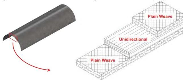
**Figure 9. Typical laminate construction for rollable tape springs.**
