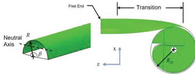
**Figure 10. Geometrics definitions of a cylindrical shell.**
