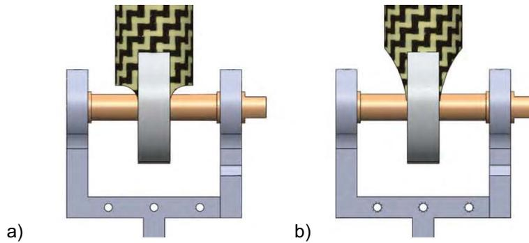
**Figure 5. Two example tape spring end clearance cuts.**
