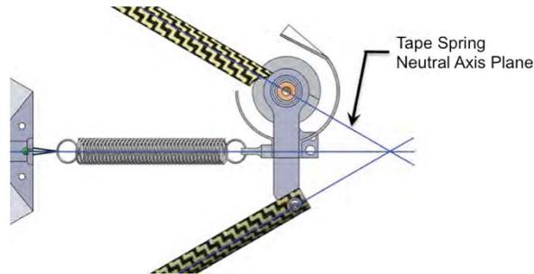
**Figure 3. Top frame tape spring neutral axes locations.**
