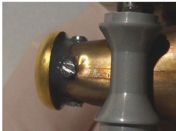
Figure 13. Tubular boom fatigue (marked in red)
