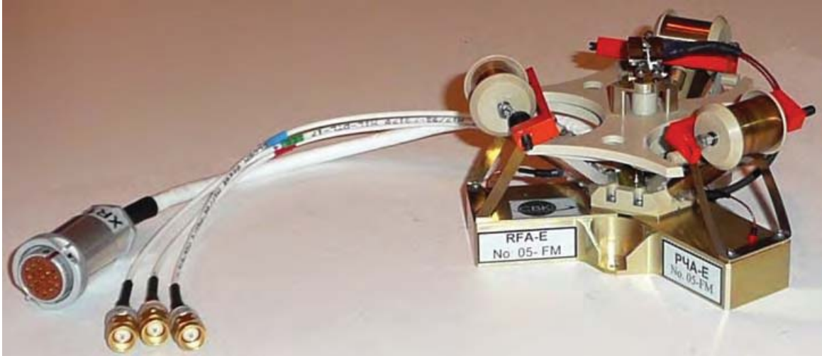
Figure 2. RFA – set of three orthogonal 1 m long antennas for RELEC mission.
