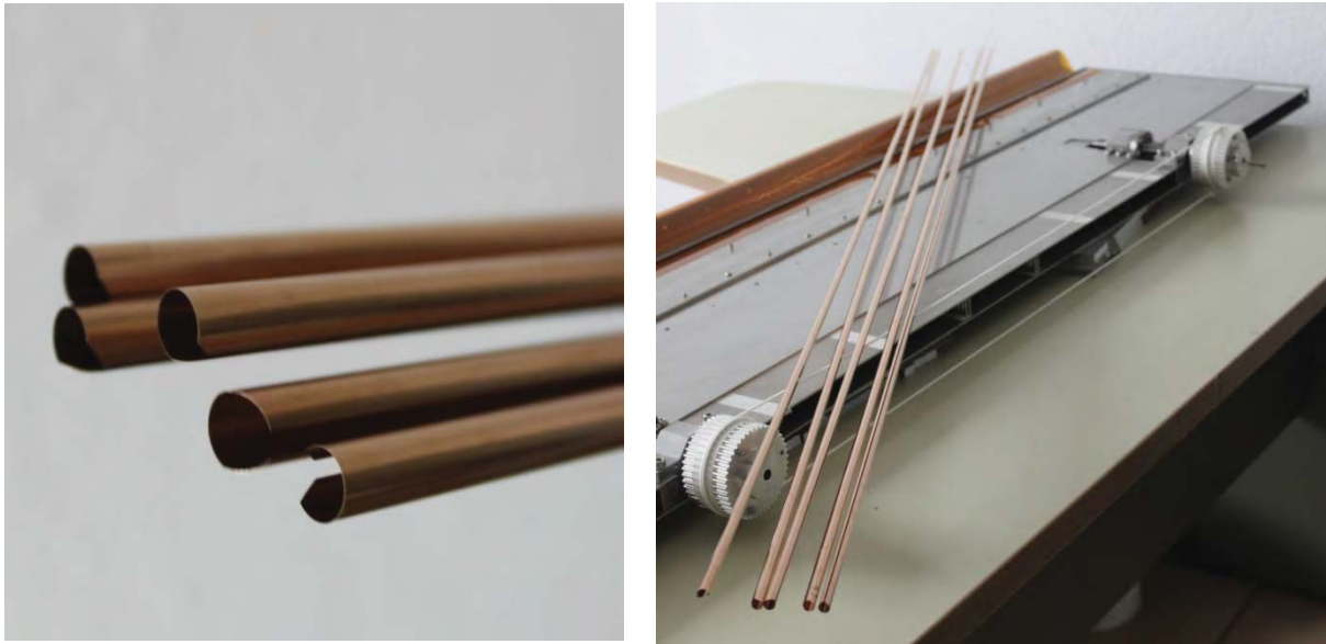
Figure 11. First series of five hardened 1.5 m long tubular booms
