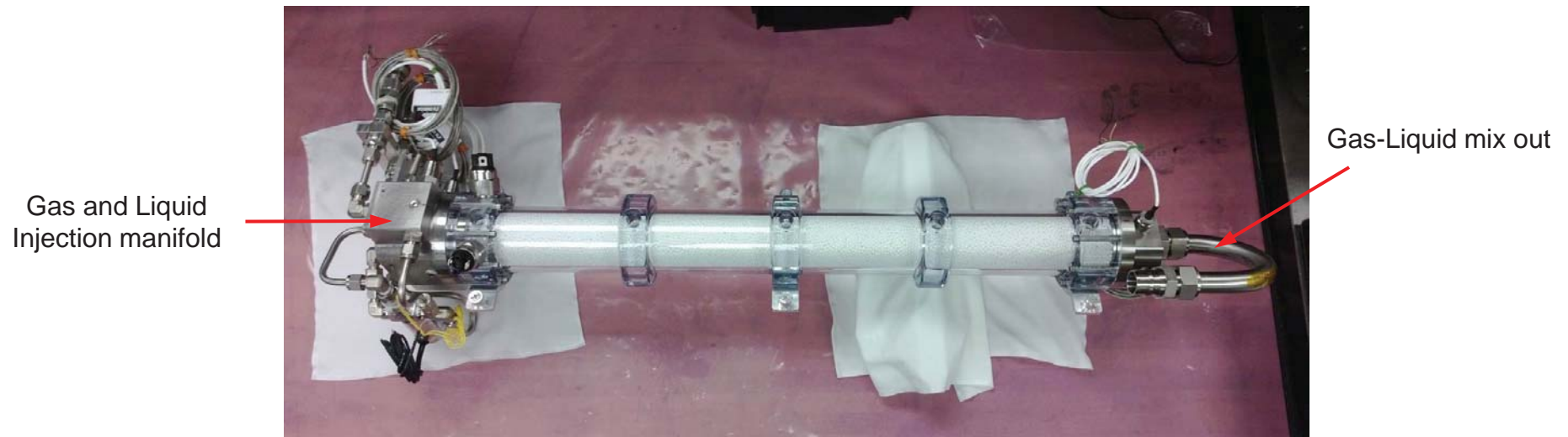
Engineering Model column packed with 3-mm Teflon beads in the ZIN fabrication area. An identical column is packed with 3-mm glass beads.
