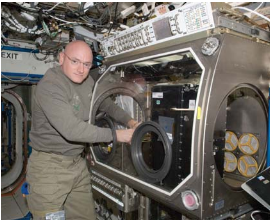
Increment 26 commander Scott Kelly installing CCF in the Microgravity Science Glovebox on ISS
