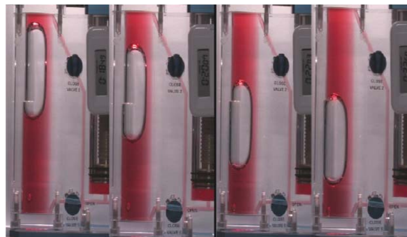
Interior Corner Flow 4 (ICF4): The snow-cone shaped test chamber includes a step change in radius along the axial direction of the test chamber. When the bubble spans the step, a pressure difference develops causing the bubble to move from the top to bottom.
