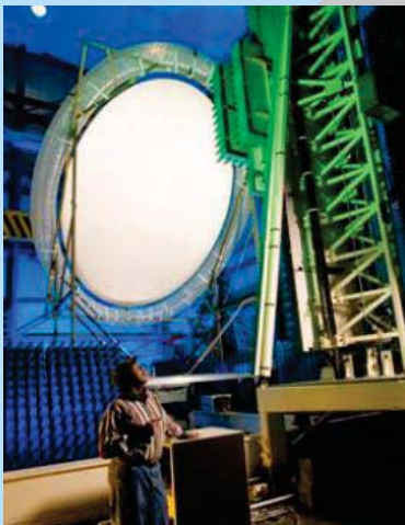
4m x 6m parabolic membrane reflector derived from solar concentrator in GRC near-field
