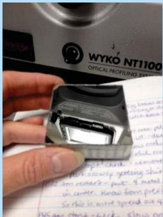
GRC/MicroEngineered Metals process developed to achieve <30 Å surface finish
