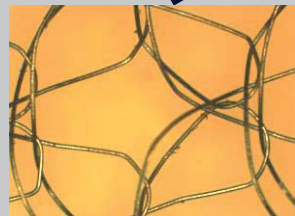
Knitted gold plated molybdenum mesh >98% reflective at Ka-band.
