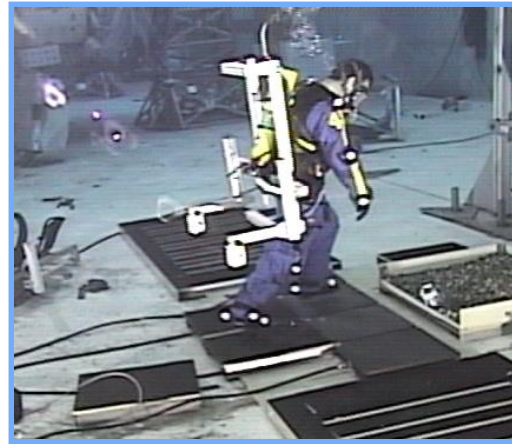
Example of a study on the effects of center of gravity on performance Neutral Buoyancy Laboratory (NBL) at the NASA Johnson Space Center
