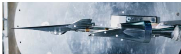
Figure 20. Photograph of X-43A stage separation interference test setup in 31-Inch Mach 10 Air Tunnel (Fig. 5 from Ref. 31).
