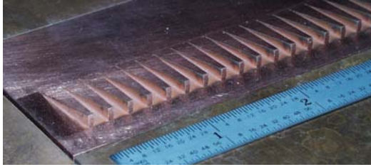
Figure 22. Final trips scaled for Mach 7 flight. (Fig. 22 from Ref. 32).
