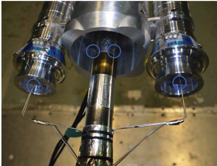
Figure 13. View of the base of the wind tunnel model with base pressure tube-ends identified by blue circles.
