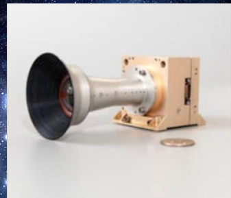
Malin ECAM M-50 NFOV (OSIRIS-Rex derived)
