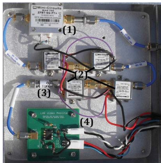
Fig. 2 The compact RF receiver amplifies and detects the beat signal that is produced in the fast photoreceiver. Components from upper right include 1 bias tee with 50 ohm resistor, 2 high-gain, low-noise amplifiers, 3 square-law detector, and 4 video amplifier
