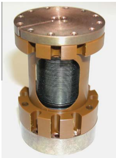
Fig. 1. Bellows-sealed gas-gap heat switch with external Vespel™ SP-1 support. The outer diameter of the top and bottom flanges are 38 mm.
