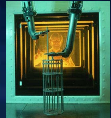
Remote manipulators within a hot cell.
