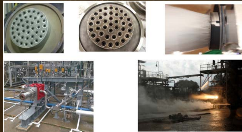
LOX/H2 SLM Injector Testing
