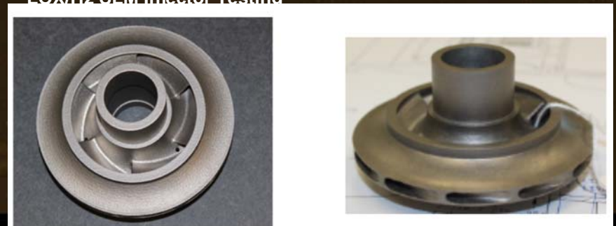
SLM Ti6-4 Turbopump Impeller
