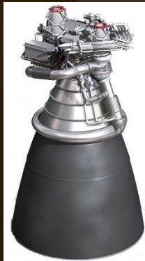
J-2X Film-Cooled Nozzle Extension (U of MD)
