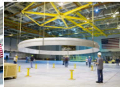
Core Stage: First full set of flight rings completed; production is underway on barrels for EM-1.
