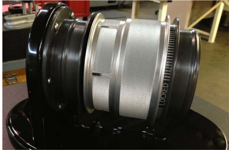
Figure 5 ISS IMV Coupling
