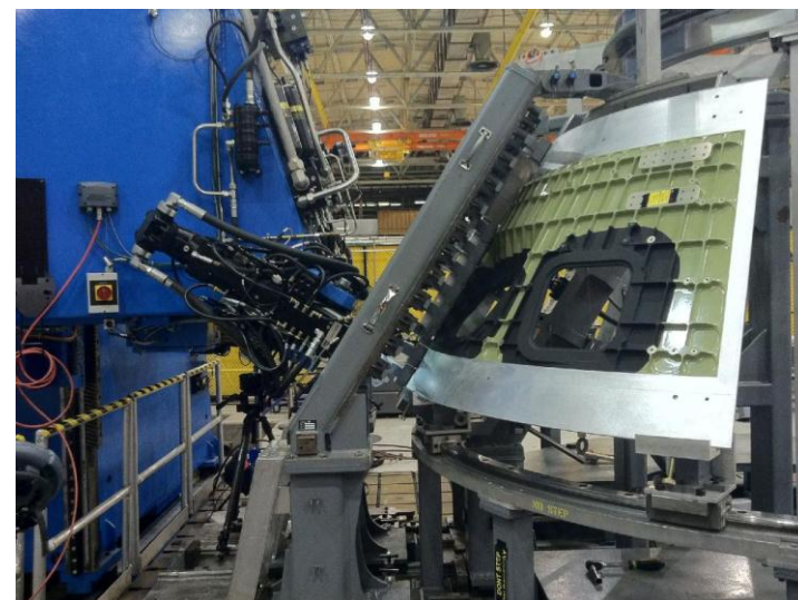
Welding of the Orion capsule at MAF. [2]
