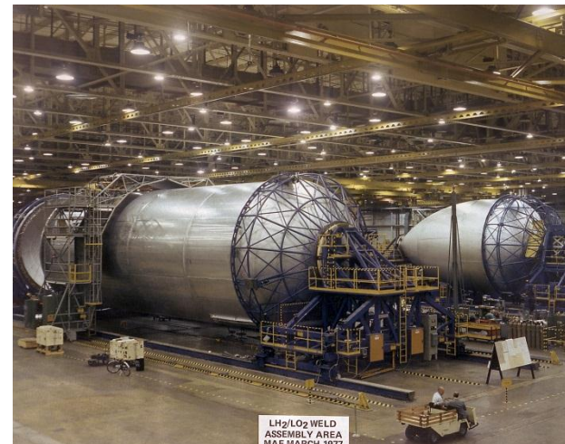
Space Shuttle External Tank major weld area. 1977
