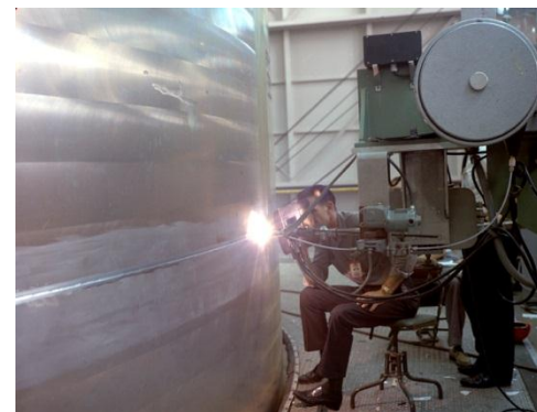
Above: Closeout welding operation of the liquid oxygen tank for the Saturn V SA-501 vehicle for the Apollo 4 mission. 1965
