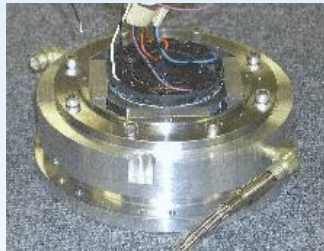
Magnetic Bearings – Used to levitate rotor. These non-contact bearings provided low loss, high speeds, and long life.
