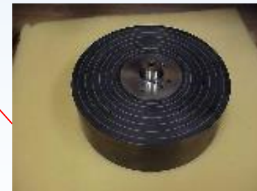
Composite Rotor – Stores energy. High energy density is achieved through the use of carbon composites.
