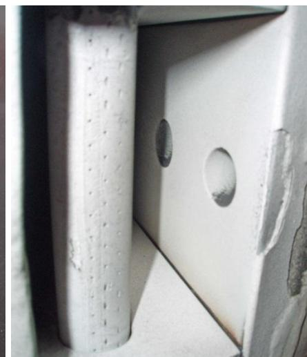
Coated CVI SiC/SiC vane after 31 hour testing at 2500°F+ coating temperature
