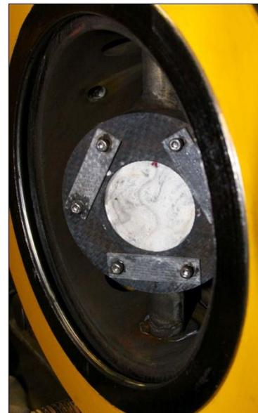
2" diameter ND3 EBC/SiC/SiC specimen after testing in the high pressure burner rig At 2600°F
