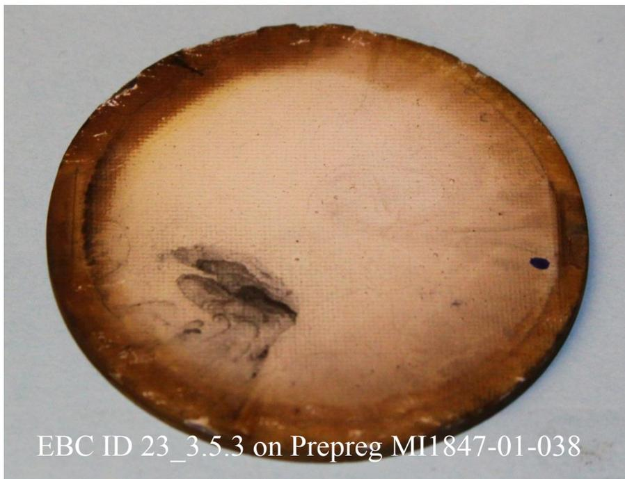
High pressure burner rig, 16 atm, 31 hr
