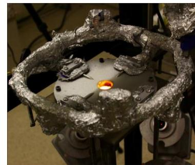
High temperature testing with steam flow
