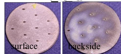
Tested 10-hole film cooled CMC specimen
