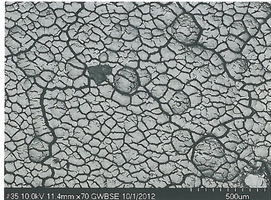
Coating Surface creep fatigue strains 1.5-2.2 %
