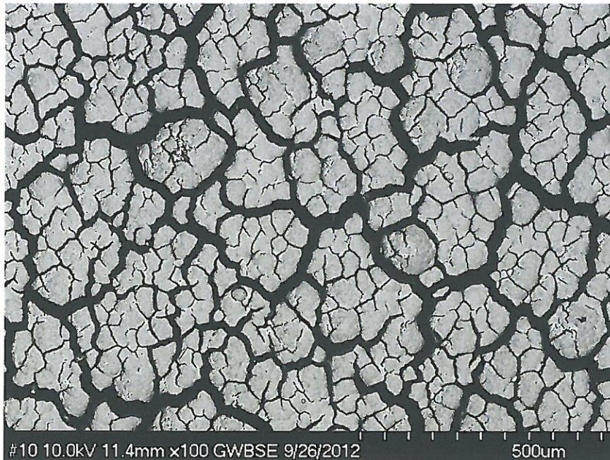
Coating Surface creep fatigue strains 6-9%
