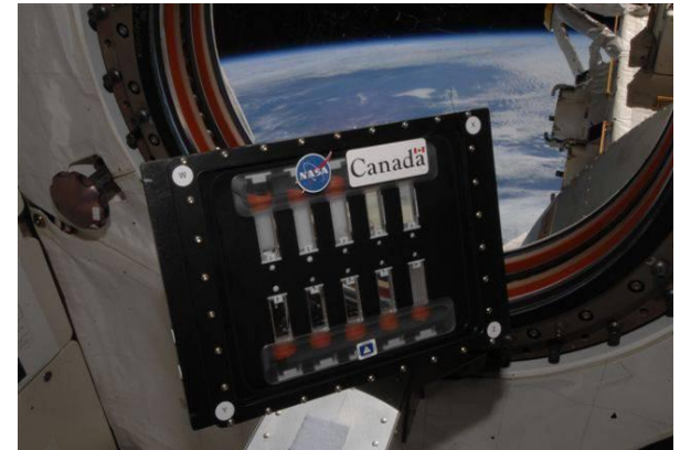
BCAT-5 colloid experiment presently on the International Space Station (ISS).
