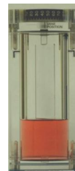
45° vane angle in earth gravity.
