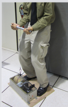
Variable Load Device NASA JSC Software Robotics and Simulation Division Device provides the equivalent of an entire set of weights in a breadbox-sized package and is capable of weight and inertia simulation and rowing-type exercises.
