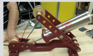
Gas Spring Device—ZIN Technologies Device primarily focuses on high load resistive exercises with a secondary focus to provide a means for aerobic exercise.
