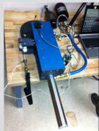
Cam Air Spring Device—ZIN Technologies Device is designed as a modular, scalable bench top unit to provide near-perfect-linear loading with a cam profile designed to produce a constant torque output from the varying piston force.
