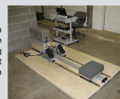
Variable Load Device NASA JSC Software Robotics and Simulation Division Device provides the equivalent of an entire set of weights in a breadbox-sized package and is capable of weight and inertia simulation and rowing-type exercises.
