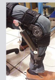
Linear Magneto-Rheologic Device NASA JSC Software Robotics and Simulation Division Utilizes an exoskeleton using linear magnetic rheological fluid dampers at the joints.
