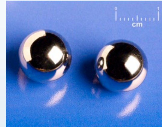
Highly polished 60NiTi bearing balls
