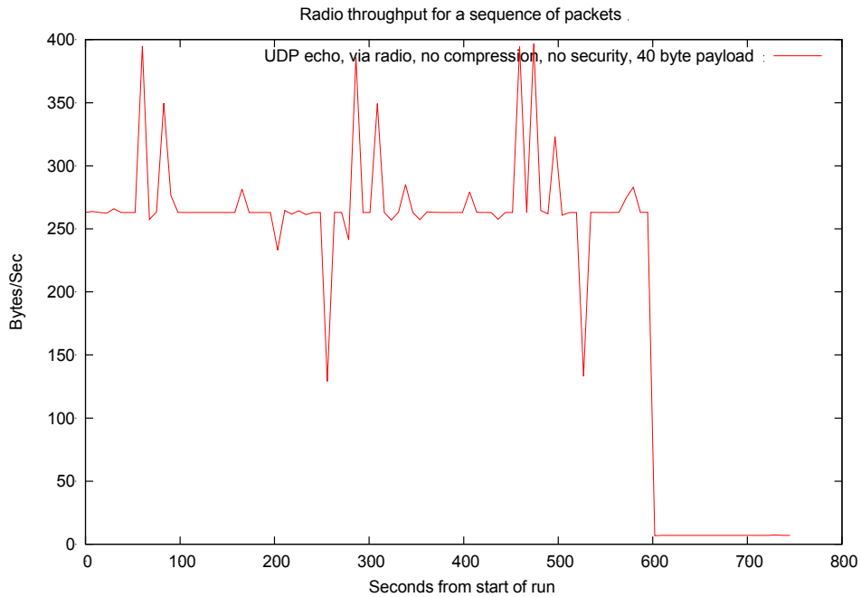
Figure 13.—Radio throughput for a sequence of packets. UDP echo, via radio, no compression, no security, 40 byte payload.
