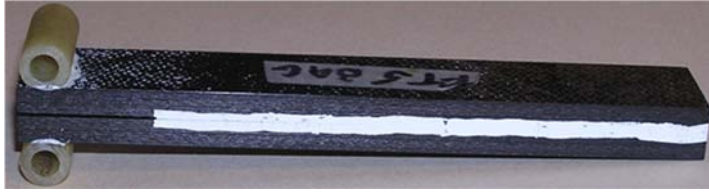
Figure 1. DCB test specimen with 2.5-inch flaw.
