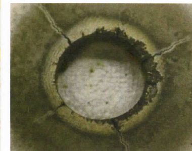
EBC-CMC specimen after 500 hr durability
