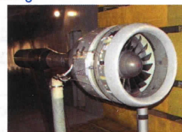
Microwave sensors installed on the NASA Turbofan Test Rig at the GRC's 9x15 LSWT
