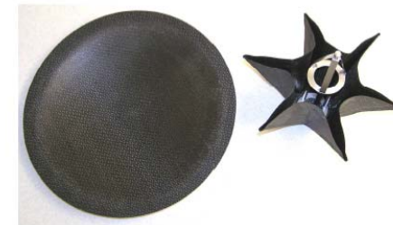
Figure 4. 0.5-m Diameter SMP Reflector in Both Deployed and Packed Configurations
