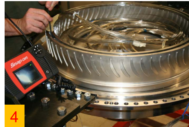
and the mating surfaces are checked for a tight fit with a boroscope
