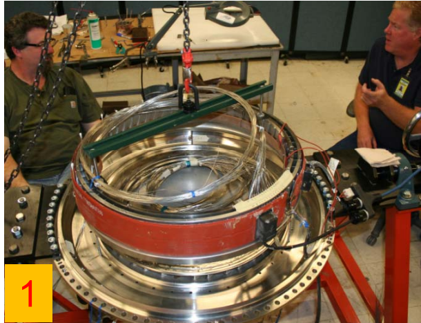
The diffuser is heated using the heating belts
