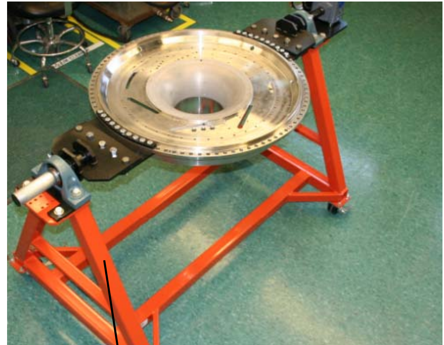
A special fixture was fabricated to assemble diffuser, EGV and shroud
