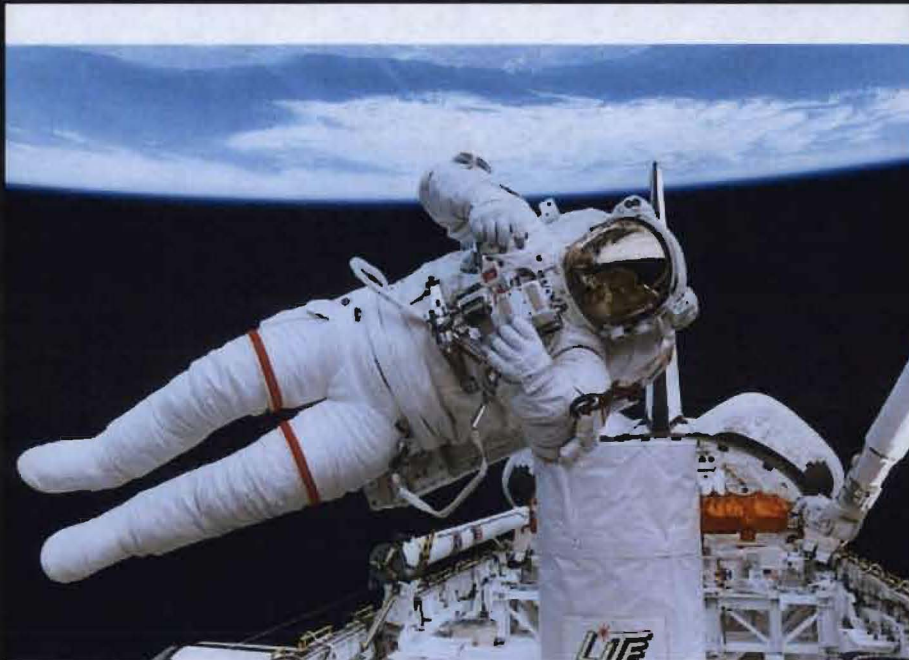
Dryden Flight Research Center EC94-42845-1 Photographed 1994 Untethered astronaut using new Extravehicular Maneuvering System (EVA) STS-64 Discovery Mission
