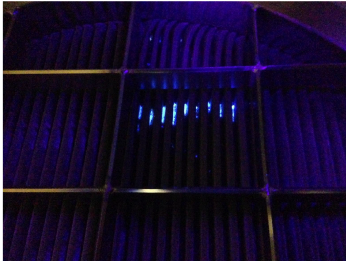
UV Illuminated Image Shows the Accumulation of Fibers in the Pleated Valleys
