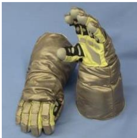
Figure 4: HPEG glove EPGs that incorporate flexible aerogel
