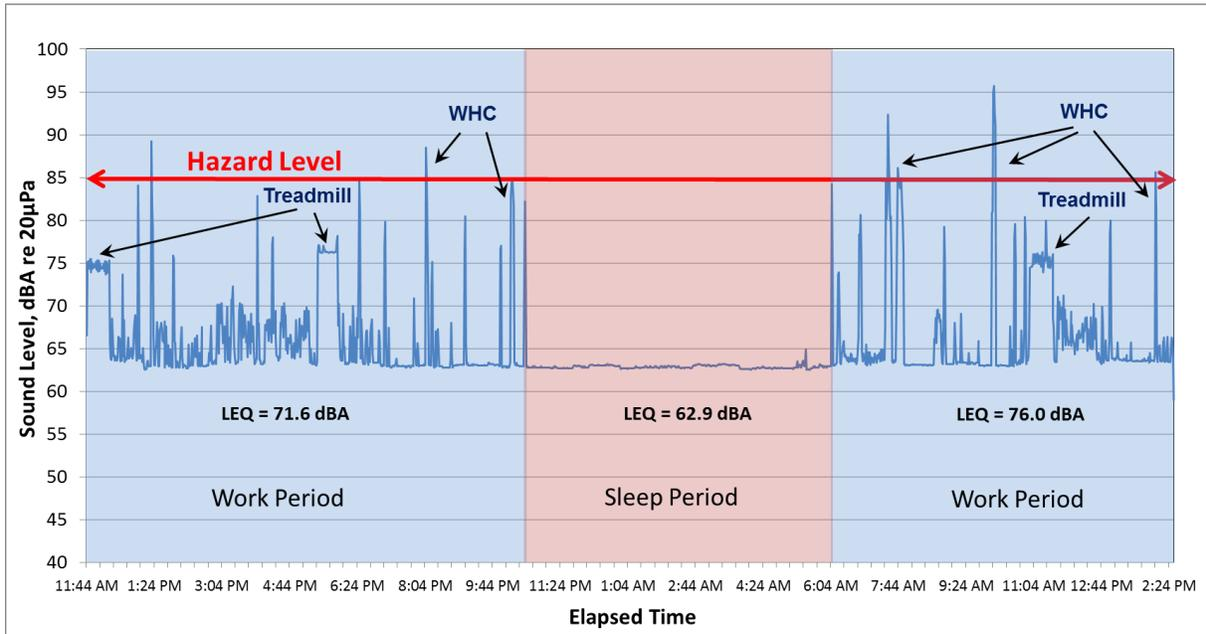
**Figure 12. Acoustic Dosimeter Static Measurement – Inside WHC, Before Pump Replacement.**
