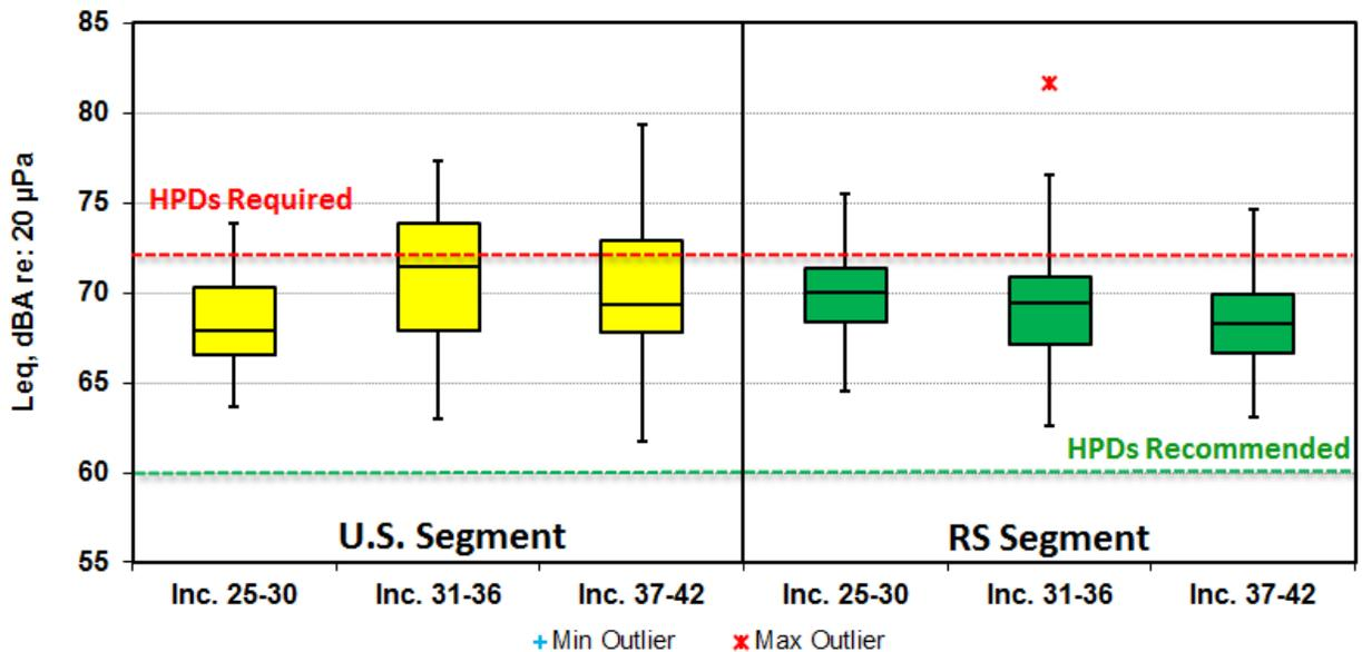
**Figure 4. Time comparison of the distribution of  $L_{EQ16}$  during work hours in the US and RS segments.**
