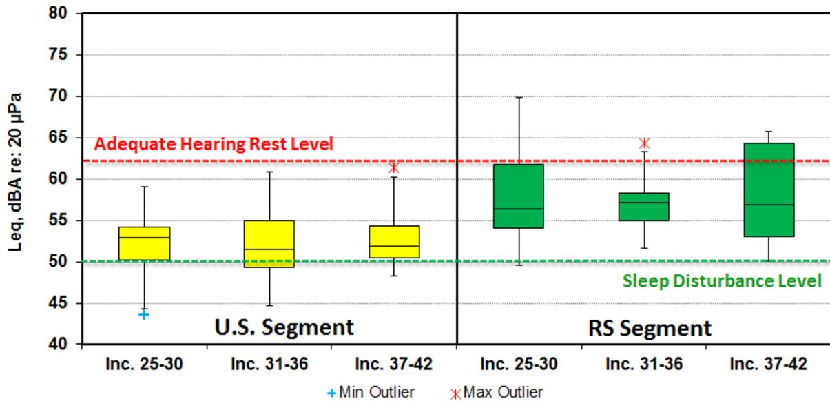
Figure 6. Time comparison of the distribution of  $LEQ_8$  during sleep time hours in the U.S. and RS segments. SOURCE: Acoustic dosimeter data collected from October 2010 (Inc. 25) through March 2015 (Inc. 42).
