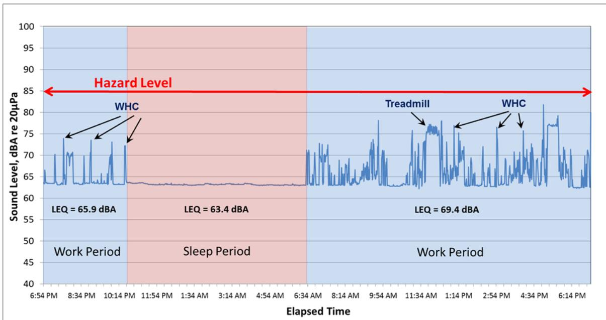
**Figure 13. Acoustic Dosimeter Static Measurement – Inside WHC, After Pump Replacement.**
