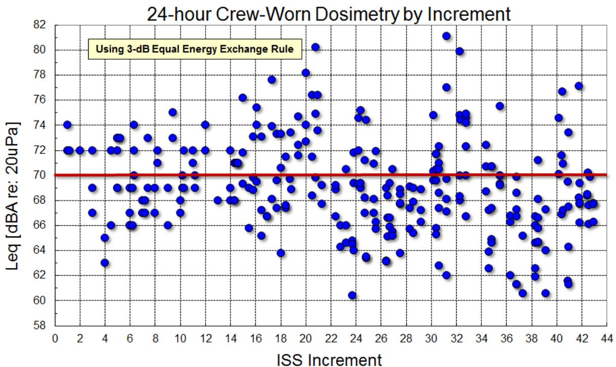
**Figure 2. 24-Hour Crew-worn Dosimetry vs. ISS Increment.**
