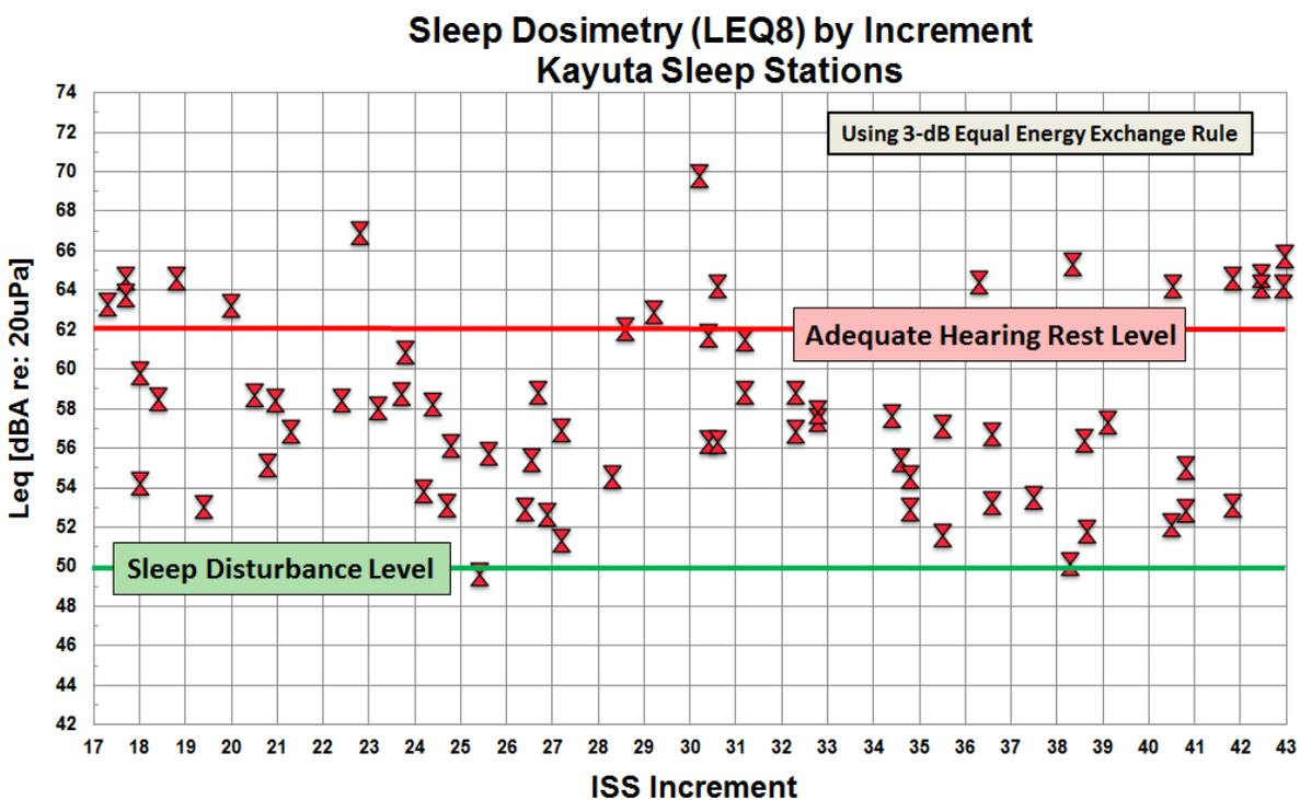
**Figure 5. Sleep Dosimetry vs. ISS Increments (Russian Segment).**
