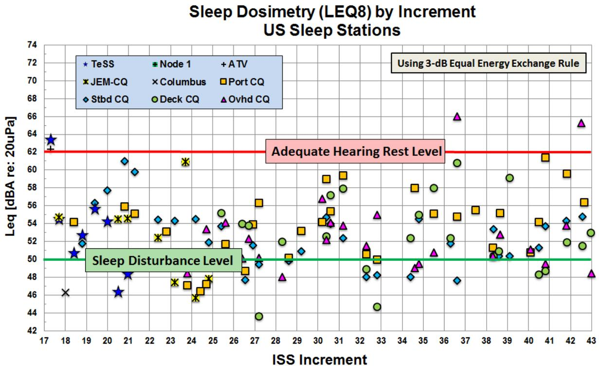
Figure 7. Sleep Dosimetry vs. ISS Increments (U.S. Segment). SOURCE: Acoustic dosimeter data collected from July 2008 (Inc. 17) through March 2015 (Inc. 42).
