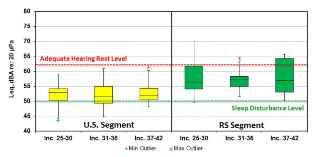
Figure 6. Time comparison of the distribution of LEQ8 during sleep time hours in the U.S. and RS segments. SOURCE: Acoustic dosimeter data collected from October 2010 (Inc. 25) through March 2015 (Inc. 42).
