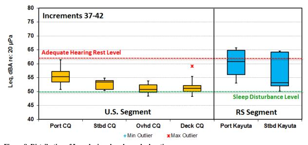
Figure 8. Distribution of  $L_{EQ8}$  during sleep hours by location. SOURCE: Acoustic dosimeter data collected from April 2013 (Inc. 37) through March 2015 (Inc. 42).
