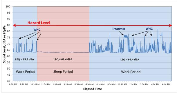
**Figure 13.** Acoustic Dosimeter Static Measurement – Inside WHC, After Pump Replacement. SOURCE: Acoustic dosimeter data collected on April 2014 (Inc. 40).
