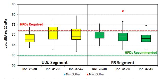
**Figure 4. Time comparison of the distribution of L**<sub>EQ16</sub> **during work hours in the US and RS segments.** SOURCE: Acoustic dosimeter data collected from October 2010 (Inc. 25) through March 2015 (Inc. 42).
