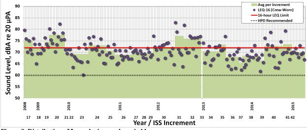
**Figure 9. Distribution of L**<sub>EQ16</sub> **during work-period hours.** SOURCE: Acoustic dosimeter data collected from July 2008 (Inc. 17) through March 2015 (Inc. 42).
