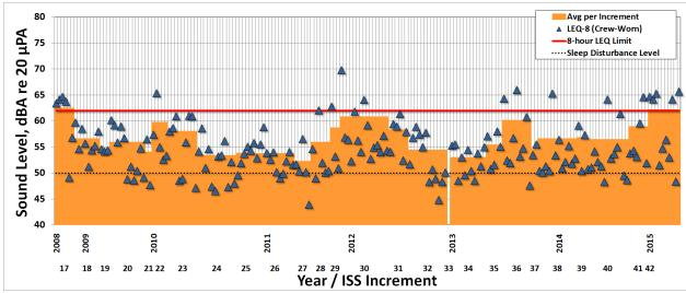
**Figure 10. Distribution of L**<sub>EQ8</sub> **during sleep-period hours.** SOURCE: Acoustic dosimeter data collected from July 2008 (Inc. 17) through March 2015 (Inc. 42).
