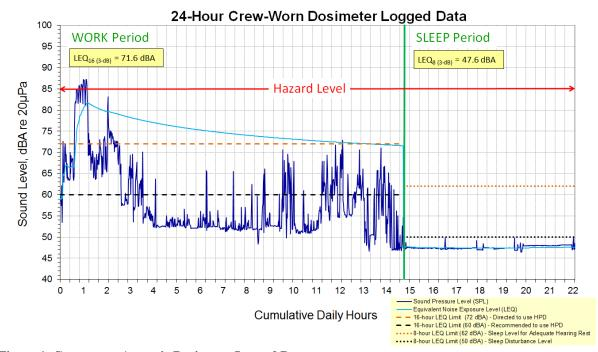
**Figure 1. Crew-worn Acoustic Dosimeter Logged Data.** SOURCE: ISS Acoustic dosimeter data collected on August 2013, Increment 36.
