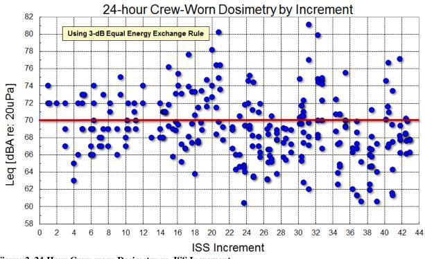
Figure 2. 24-Hour Crew-worn Dosimetry vs. ISS Increment. SOURCE: Acoustic dosimeter data collected from November 2001 (Inc. 1) through March 2015 (Inc. 42).
