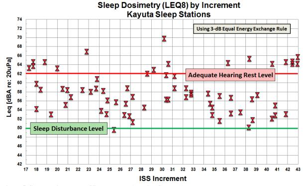
**Figure 5. Sleep Dosimetry vs. ISS Increments (Russian Segment).** SOURCE: Acoustic dosimeter data collected from October 2010 (Inc. 17) through March 2015 (Inc. 42).
