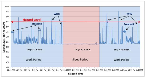
the source for the high noise levels. The pump was then replaced and the levels returned back to nominal levels. At that point, the WHC was then removed from the NHI (See Fig 13).
