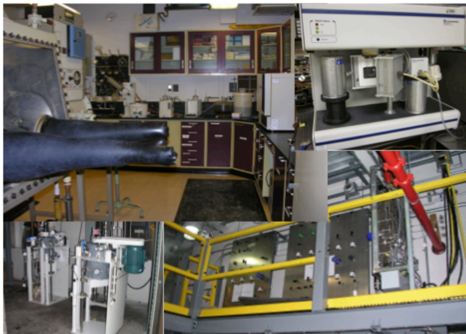
Figure 3. Example facilities for processing catalysts, characterizing, and screening fuel production catalysts; from upper left-hand corner: synthesis laboratory, instrument for TPR analysis, Alternative Fuel processing Facility, and continuously-stirred tank reactor.
