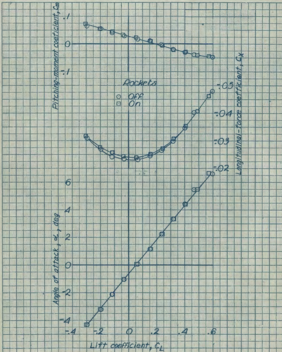
Figure 32.- Effect of rockets on the aerodynamic characteristics in pitch of the 1/5-scale model of the Republic XP-84 airplane with revised horizontal tail. \alpha = 0^\circ .
