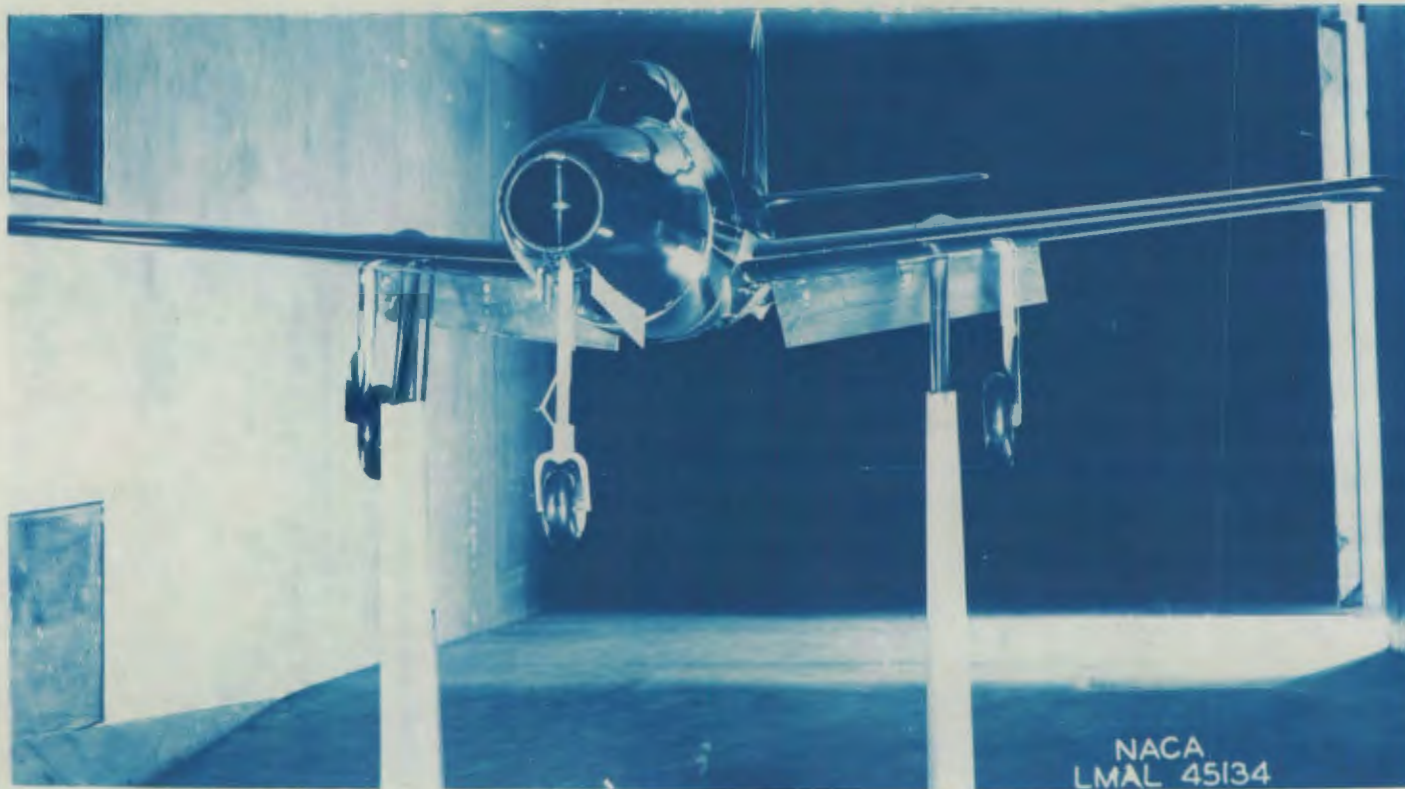
Figure 3.- The \frac{1}{5} -scale model of the Republic XP-84 airplane (Army Project MX-578) mounted in the 300 mph 7- by 10-foot tunnel.
